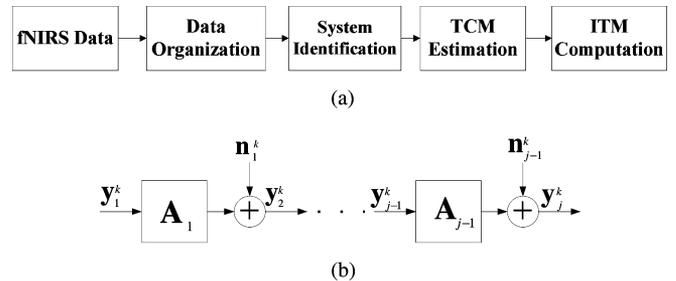
Fig. 1. General description of the proposed setup. (a) Block diagram of the system. (b) Diagram of proposed AR-1 model.
